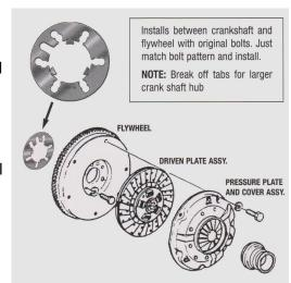
\*NOTES: The shim pictured "Full Sized" below can be used to make sure you select the correct shim. Just print these instructions and match hole pattern to flywheel. Be sure your printer is set to "No Size/Scale Change". You can check for correct scale by matching the ruler on the page.
