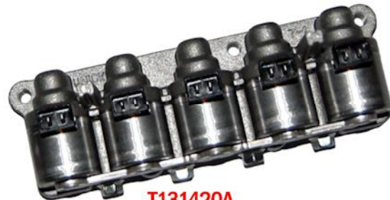
T131420A SOLENOID 5 PACK Fits '06-up A4CF1 / A4CF2 (3.0-3.4 Ohms)
