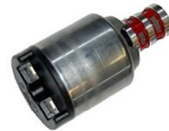
T41435A LATE KM VFS SOLENOID Fits '05 up F4A41/42/4B/51, F5A51, A5HF1/GF1 (4.0-4.7 Ohms)
