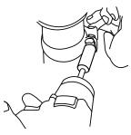
Align the two flats to the bolt and attach the new hardware on each side with the appropriate wrench or tool.
