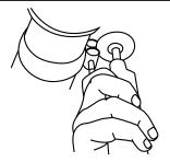
To repair the worn hardware, simply cut the existing clamp in the middle until the bolts fall off.
