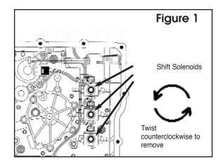
**1. To Remove:** Depress the spring tab and twisting the solenoid to the left until it clicks **(Figure 1)**. Pull the old solenoid from the valve body.
