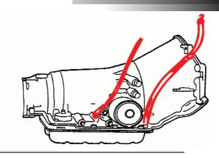
NOTE: This is definitely NOT a bolt-in Kit because the overall length will increase by 1 7/8". Be prepared to either reposition the engine or alter the drive shafts and shifter hole to compensate for the added length of the rebuilt unit.
