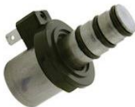
K41954 LATE KM SOLENOID Fits '98-up F4A41/42/48/51, A5HF1, R4A51, R5A51, V4A51, V5A51, W4A42 All positions except VFS position in '05-up units (2.6-3.4 Ohms) Genuine OEM Part 46313-39051
