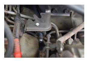
The longer bracket is used to attach the inner wire end to the accelerator bracket.
