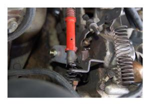
You may find it easier to attach the cable head to the first bracket before installing as it is a tight fit. Once the cable head is installed into the first bracket the inner cable end can be attached into the connector on the installed long bracket.
