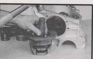
Install the Teckpak/Fitzall Stabilizer bearing.
